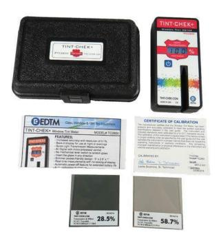
the unit up and similarly to the Tint-Chek is not affected by ambient light. The meter comes in a hard-sided carrying case designed to protect the unit in hostile environments. Along with the meter, the Tint-Chek + case includes a User Manual and Certificate of Calibration, guaranteeing that the
