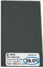
Light Transmitted through the standard is recorded on the testing standard and is written on the bottom of the glass sample. To test the accuracy of your meter simply clean the test sample with a micro-fiber cloth and follow the steps that were demonstrated above by inserting the testing sample in place of the window. Your readings should be within +/-2% of the number listed on the test sample if your Tint-Chek is operating at factory performance level.
