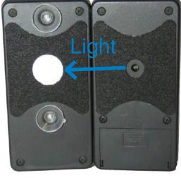
wavelengths in the visible range. The center of this range is about 550nm. Your meter does this by firing a high energy LED (light-emitting diode) and comparing the initial calibration value from the LED to the value
